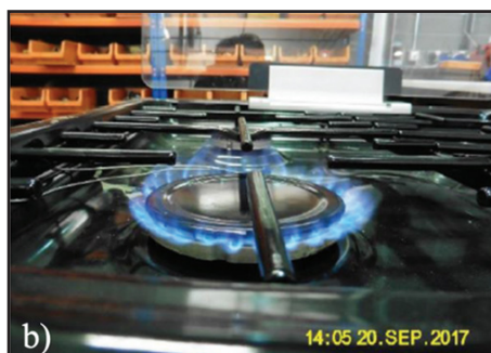
FIGURE 4 a) 100% Methane Flame; b) 28.4% Hydrogen Blend Flame [Issaac, 2019]
